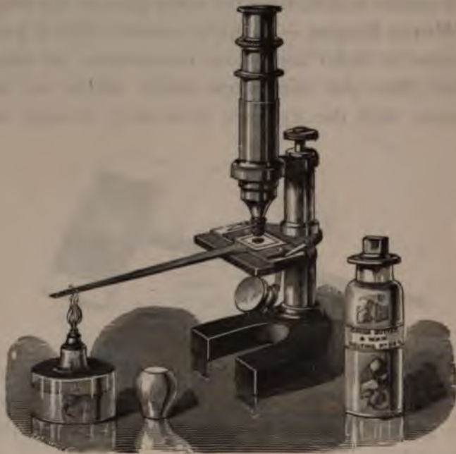
FIG. 32.—SIMPLE WARM STAGE SHOWN IN OPERATION.
